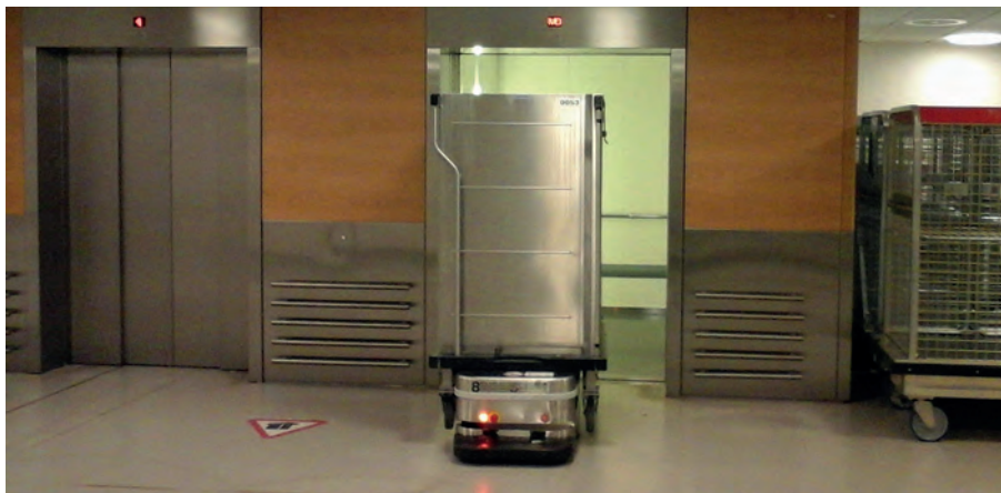
An automated guided vehicle (AGV) transporting a piece of equipment in a Norwegian hospital. Photos: Caroline Lloyd.
