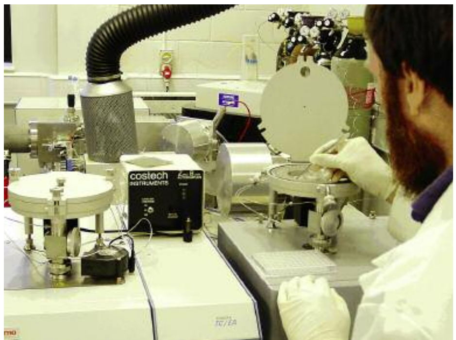
Figure 2: Prepared oxygen isotope samples being loaded into the mass spectrometer in the Department of Earth Sciences, Durham University
